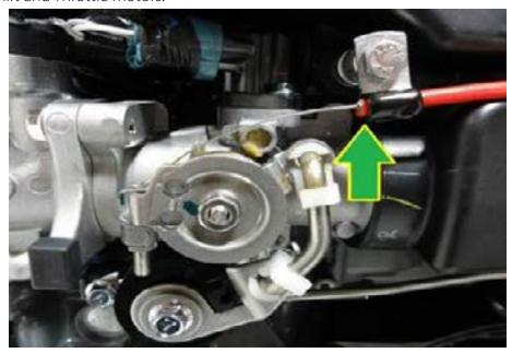
6. Attach cable loop as shown.
