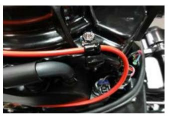
8. Mount the servo bracket as shown using the factory screw and small spacer provided in the TrollMaster kit. Please note: Make sure the small spacer is installed under the servo bracket before tightening screw.
