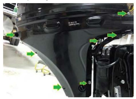
2. Remove the cowling's rear latch pin and latch.
