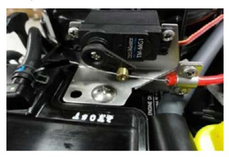
10. With the throttle closed, pull the cable tight to remove any slack, be sure the throttle remains closed. When the cable is tight, slide the crimp over the cable and crimp it tight as shown in the photo. You can then cut off the excess cable.
