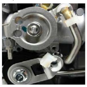
13. Install the TrollMaster cam and reinstall the factory rod & rod retainer as shown. →
