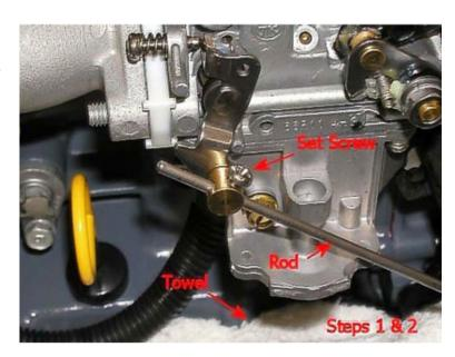
3. Do not disconnect the throttle cable. Remove the bolt in the center of the throttle cable drum.
