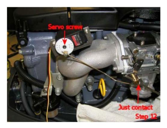
12. The factory Shift or Tiller will be out of adjustment. This is due to the change in distance between the cable drum and the carburetor and can be adjusted by loosening the set screw at the brass fitting on the carburetor. Then place the shift lever or tiller handle to the neutral/start setting and tighten the screw.
