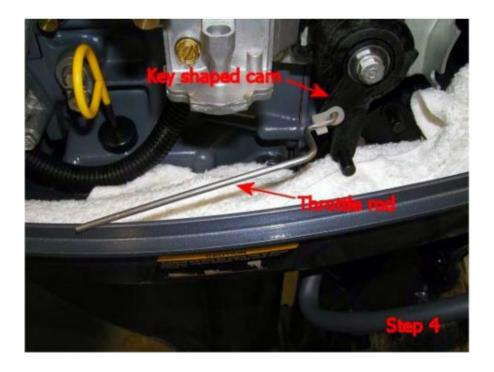
5. Remove the throttle rod from the rod retainer.
