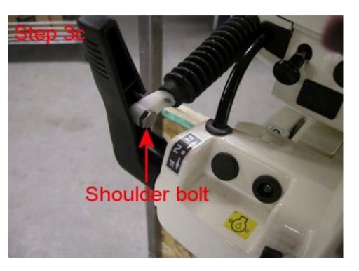
d. Disconnect the shift rod from the shifting mechanism at the nylon retainer.
