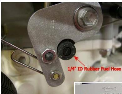
9. Using a #6 metric Allen wrench, loosen these bolts a sufficient amount to allow the servo mount bracket to slide between the bolt head and the flat washer.
