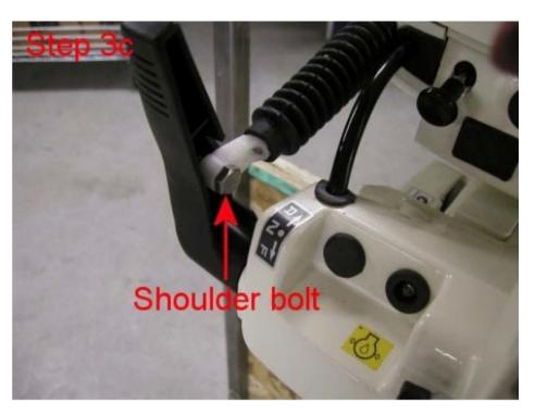
d. Disconnect the shift rod from the shifting mechanism at the nylon retainer.
