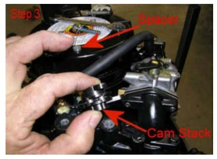
4. Install the replacement throttle rod in the carburetor fitting.
